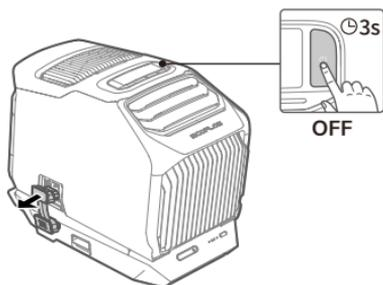
1. Power off and remove the plug
