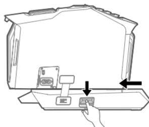
2. Press and hold the unlock button, and slide it backward
